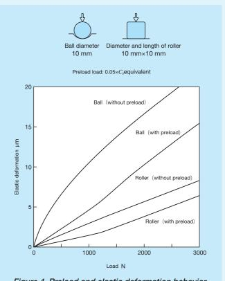
Figure 4 Preload and elastic deformation behavior
