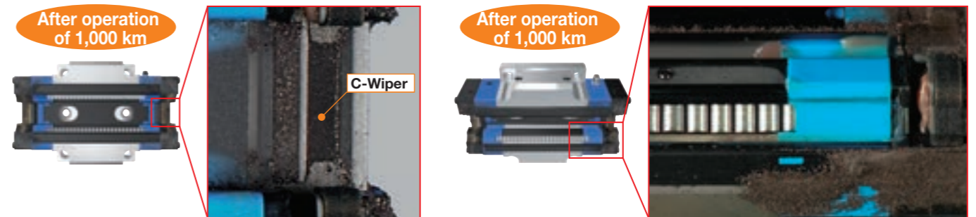
Only few foreign substances may get into the slide unit.
