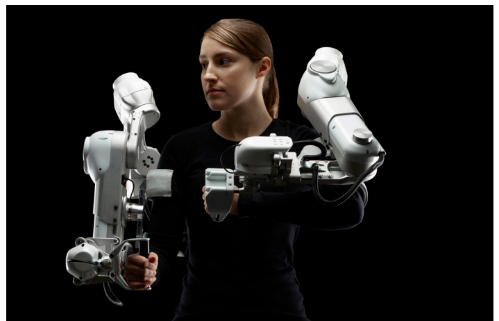
Figure 2. IKO Crossed Roller Bearings carry high moment loads in a physical therapy exoskeletal robot that helps stroke patients relearn shoulder movement.
