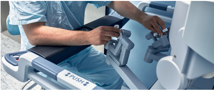
Hoop-type inputs impose different loads onto the bearing with the surgeon's various gestures, requiring a bearing that can handle radial, thrust and moment loads at the same time.
